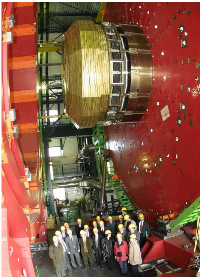
Fig.1. Overall view of the Compact Muon Solenoid (CMS). Weight 14500 ton, outer diameter 14.60 m, length 21.60 m, solenoid magnetic field 4 T. The insertion shows the systems whose construction Russia and Dubna member states (RDMS) CMS collaboration is responsible for. JINR bears full responsibility for Endcap Hadron calorimeters, HE, and Forward Muon Stations, ME1/1, and participates in Preshower, ES.
