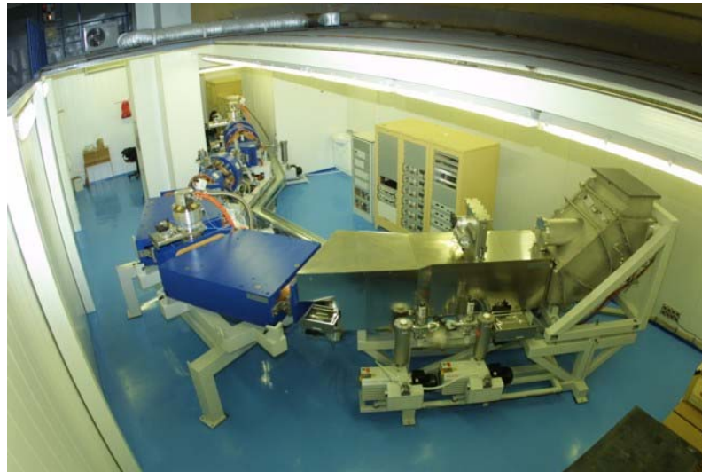
Mass Analyzer of Super Heavy Atoms
