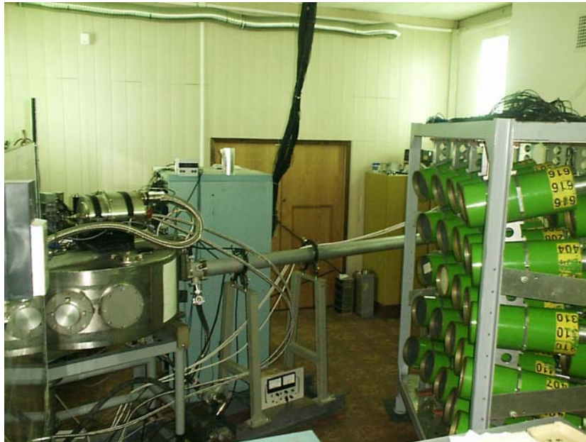
Cryogenic target array and neutron spectrometer DEMON
