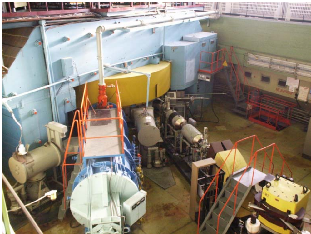
General view of the isochronous cyclotron U-400
