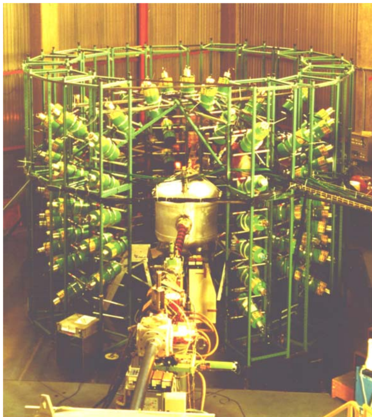
Multidetector neutron spectrometer DEMON
