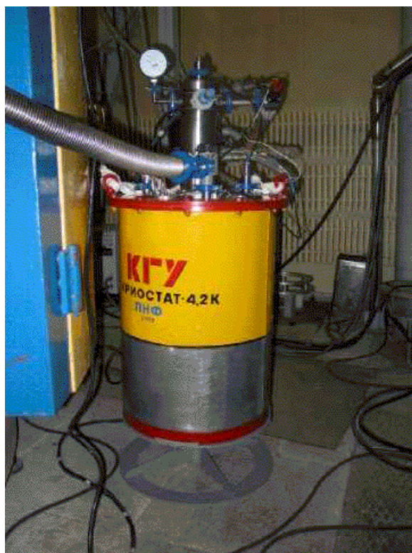
Fig.2. Closed cycle cryostat KGU801 on the basis of two-stage cryogenerator RGD1245.
