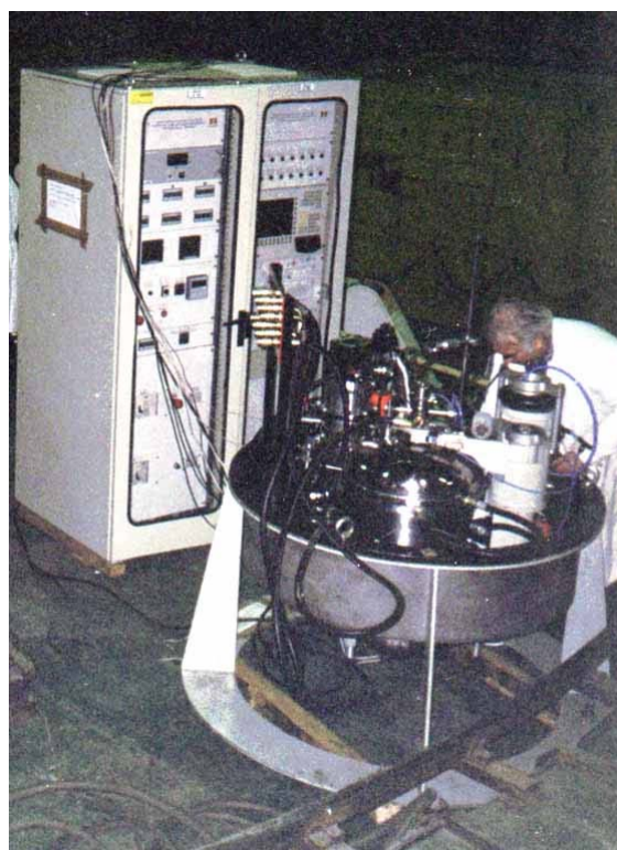
Fig.3. Thermostatic system TS-3000 to study samples at the DIN-2PI spectrometer at temperatures up to 3000 K.
