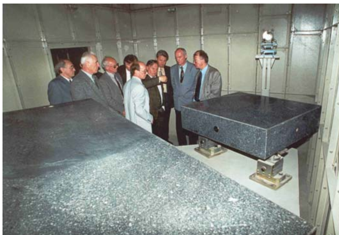
General view of an optical bench made of marble in the room of energy-dispersive EXAFS-spectrometer.
