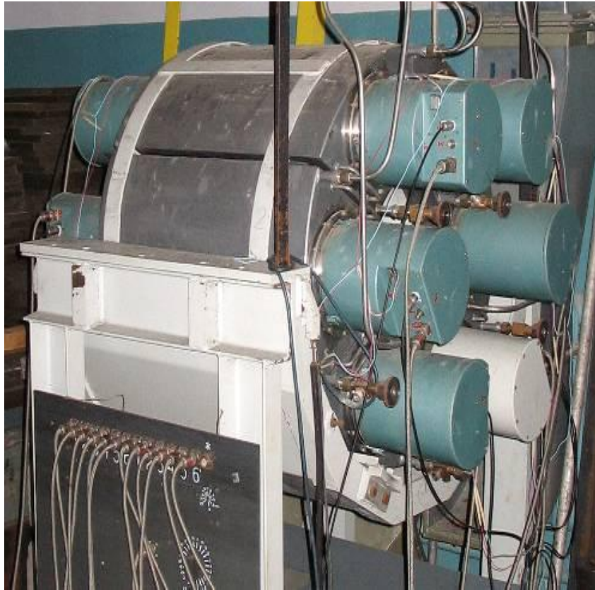
Liquid scintillator detector Six 35 L sections Electronics which is able to work at different multiplicities of gamma quanta 60 m flight path
