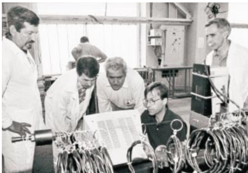
JINR Experimental Workshop. Area for testing minidrift chambers purposed for physics research at the Tevatron in Fermilab (USA) within the ДØ project
