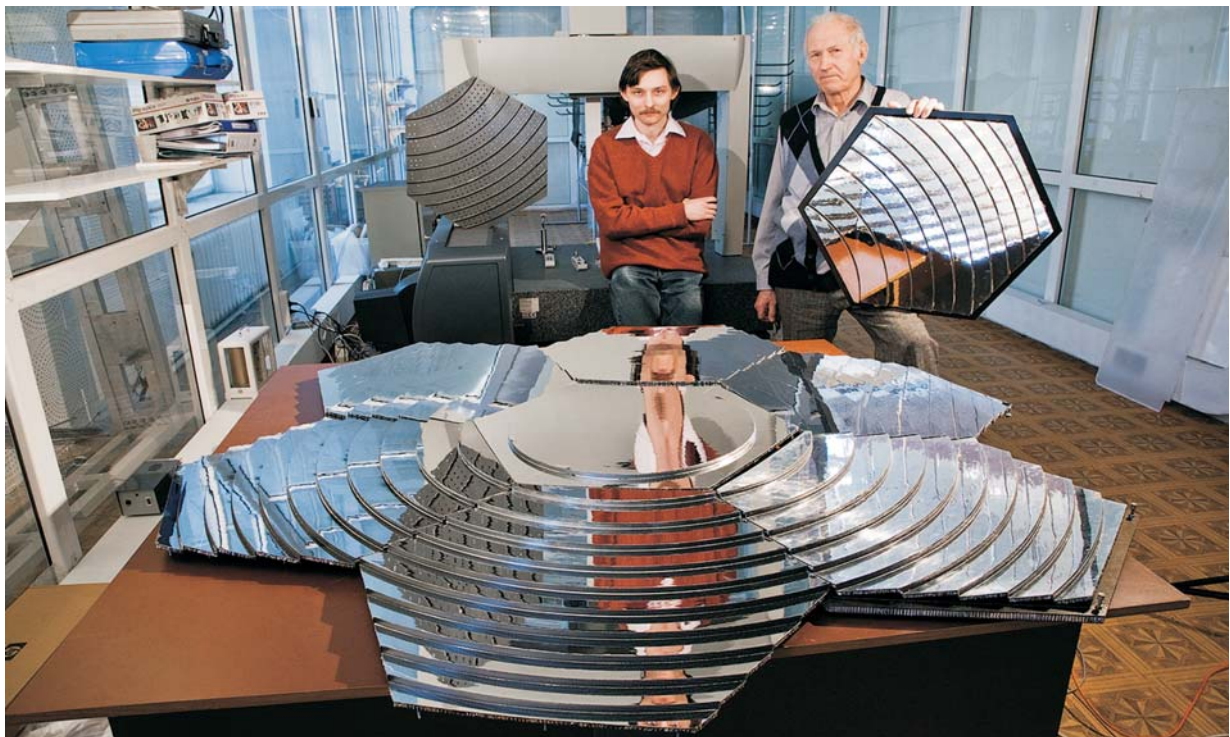
Dzhelepov Laboratory of Nuclear Problems. A technological sample of the focusing mirror for work in open space, developed at JINR in the framework of the space experiment TUS
