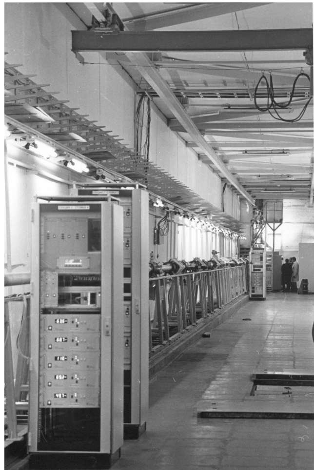
Flerov Laboratory of Nuclear Reactions. Channel of the Radioactive Beams Accelerator Complex, which links U400M and U400 cyclotrons
