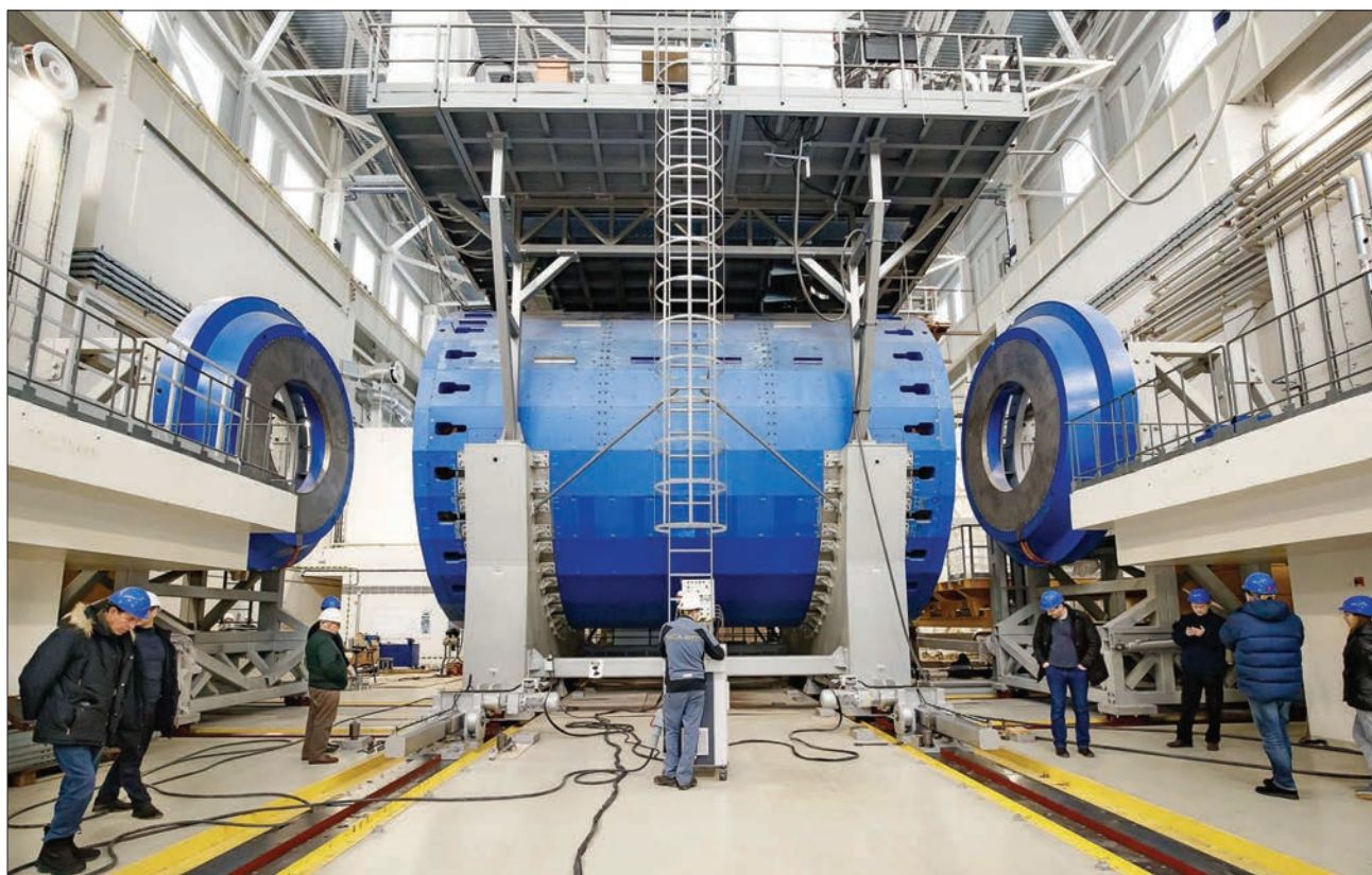
The Veksler and Baldin Laboratory of High Energy Physics, 5–6 December. A technological transfer of the 800-ton MPD experiment solenoid in the pavilion of the multipurpose detector of the NICA Accelerator Complex
