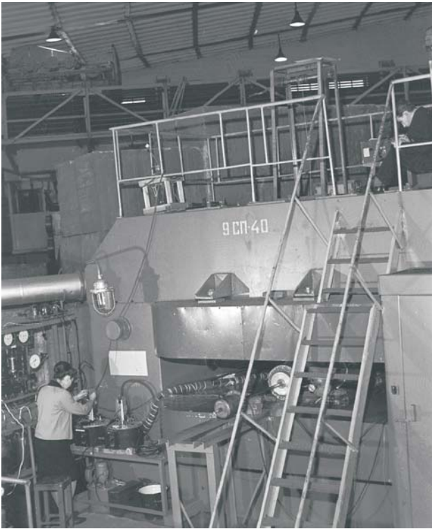
Laboratory of High Energies, December 1963. The propane chamber. Photo by V. Shustin
