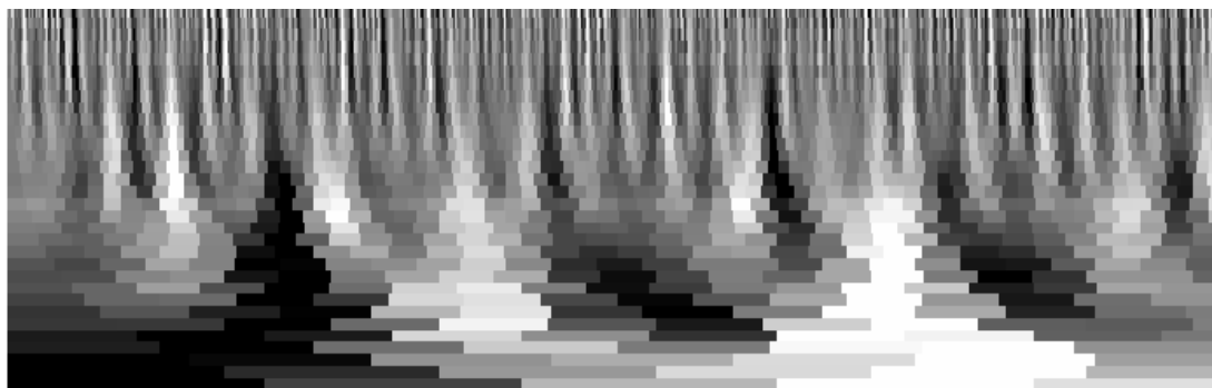
Grey shade plot of wavelet coefficients calculated for the M-segment RNA gene of the Dobrava virus primary structure. Sequence number is GI:3970669. A fragment of the first 1024 base pairs from the beginning is shown. Each layer in vertical direction corresponds to the scale base 2^{1/4} . Copied from the monograph, see below
