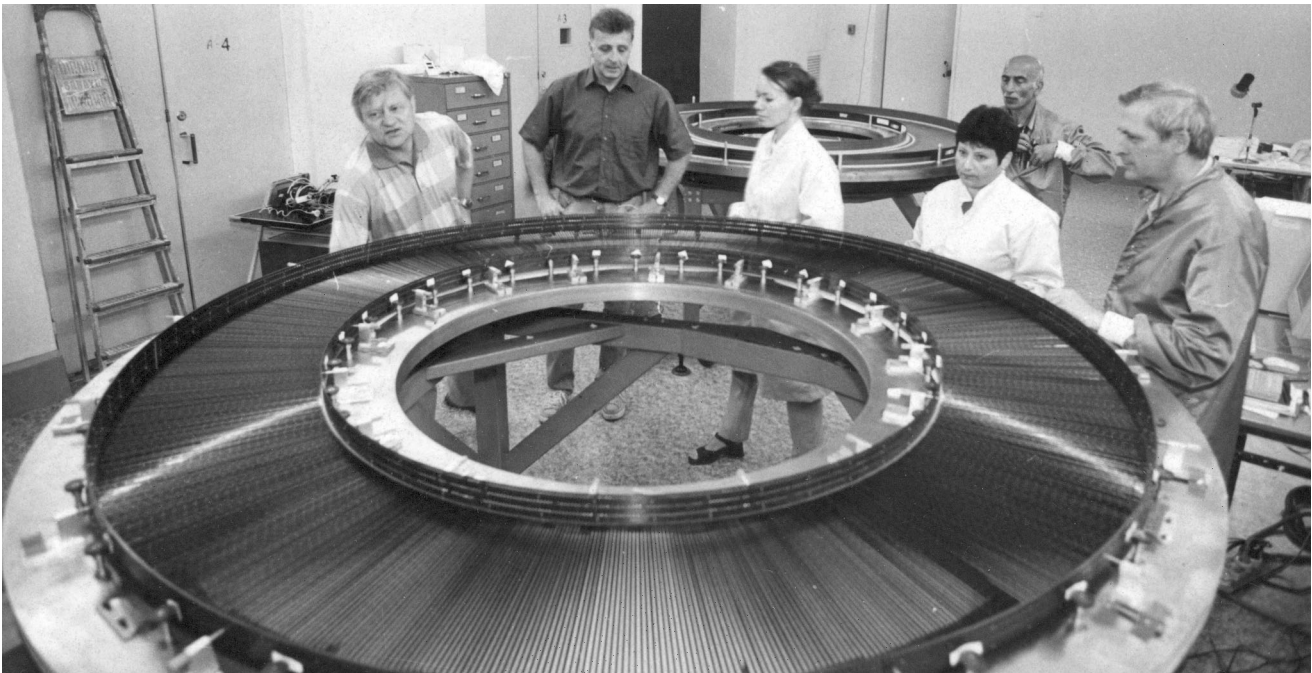
Laboratory of Particle Physics. The first ring in the mass production line of the inner detector for the ATLAS facility
