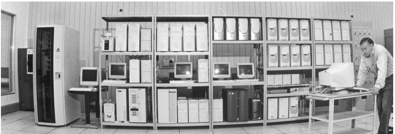
Laboratory of Information Technologies. A complex of PC clusters, consisting of an interactive cluster and computer farm of general purpose, a computer farm for the LHC (CMS, ATLAS, ALICE) experiments and a cluster for parallel counting on the basis of MYRINET technique
