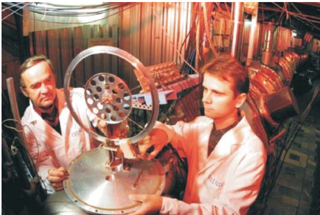
The general view of the internal target mechanism before the installation into the Nuclotron vacuum chamber
