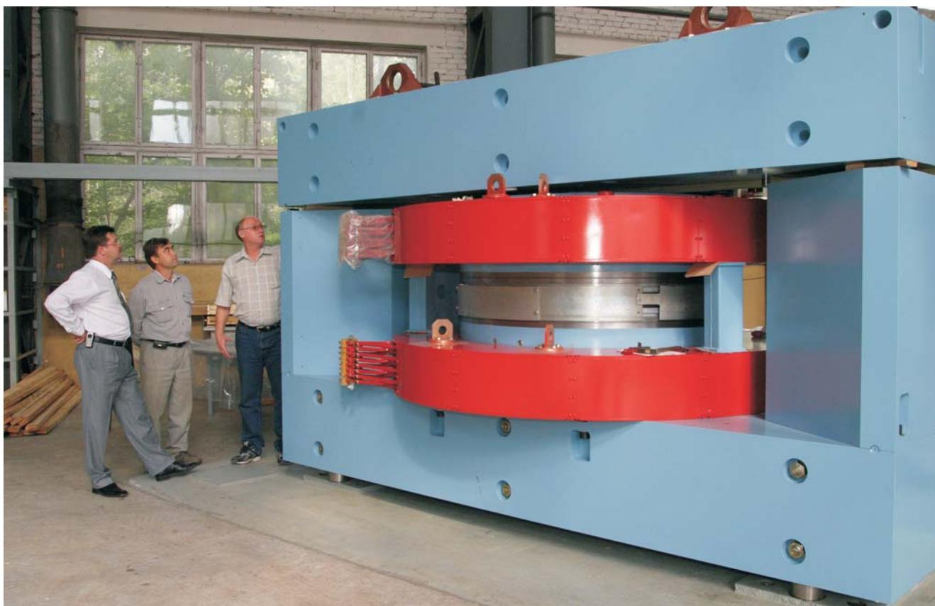
Dzhelepov Laboratory of Nuclear Problems, building 5. DC-60 cyclotron electromagnet, worked out at FLNR for Kazakhstan, at the final stage of assembling
