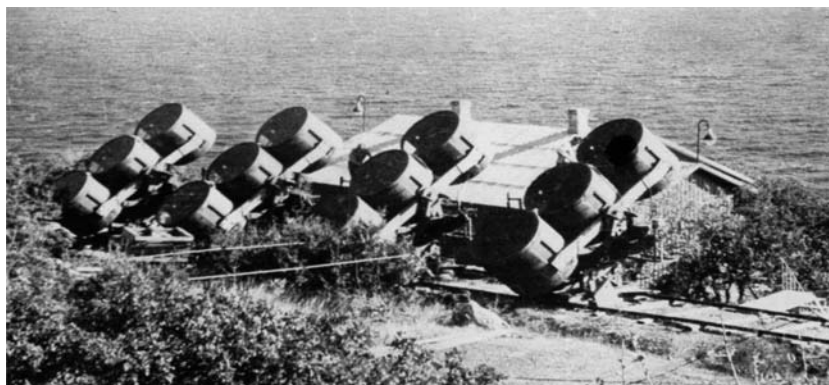
Fig. 3. The first gamma telescope in the world developed by A. E. Chudakov and his team in Crimea, USSR [10]
