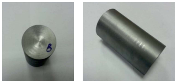
Fig. 3. Finished chromium bars after HIP
