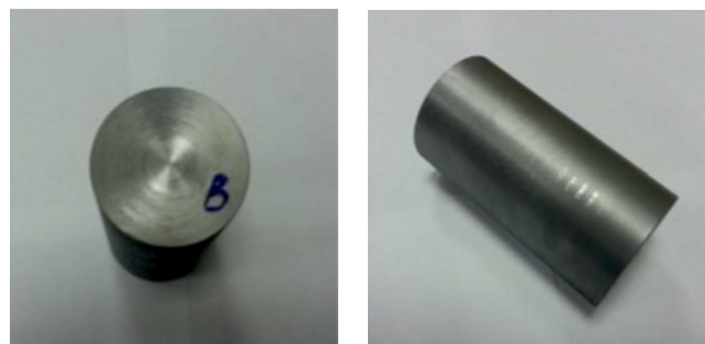
Fig. 3. Finished chromium bars after HIP
