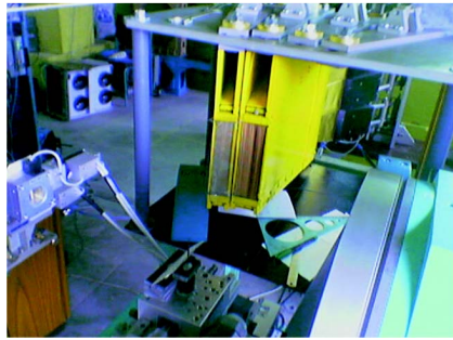
Fig. 4. Multisection radial collimator system installed on FSD rendering spatial resolution of 2 mm with the current 7 and 10° radial collimator modules
