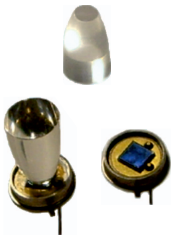
Fig. 7. View of the MAPD with and without the Winston cone
