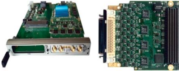
Fig. 7. Left: the example of FPGA board; right: the example of FMC card
