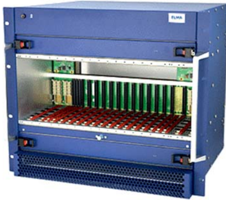
Fig. 6. MicroTCA4 crate with 12 slots PICMG
