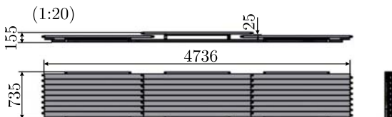
Fig. 3. The MCORD modules consist of three sections, eight scintillators each
