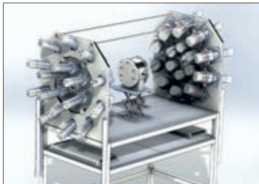
Position-sensitive TIC for PFN emission study in combination with 32 liquid scintillators
