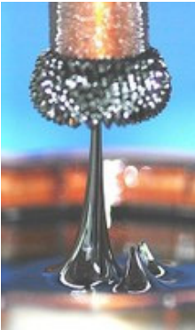
Ferrofluid under the effect of the magnetic field of a simple electromagnet
