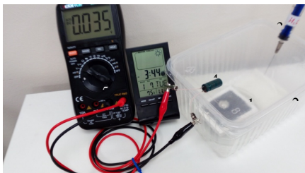
Fig. 2. Measuring cell, where: 1 - sample of a chemo-electric converter; 2- humid air chamber; 3- syringe with distilled water; 4- electric capacitor 2200mkf x 6V.
