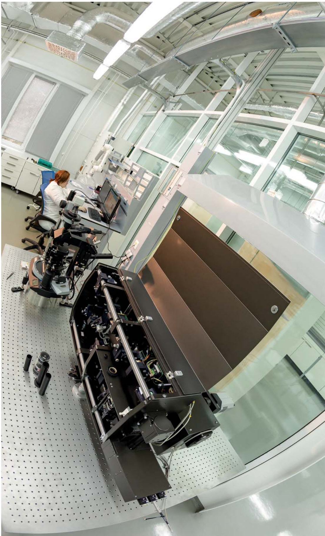
The Flerov Laboratory of Nuclear Reactions. The scanning probe microscope for profiler measurements NTEGRA Spectra
