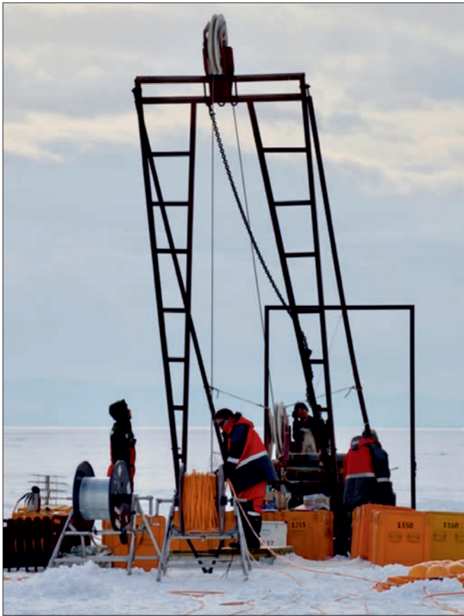
Baikal, April. Deep-underwater assembly of a garland of the neutrino telescope Baikal-GVD
