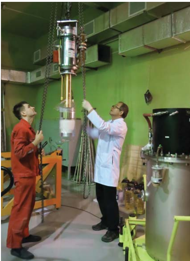
The Frank Laboratory of Neutron Physics. Assembling of new modulators for the IREN facility
