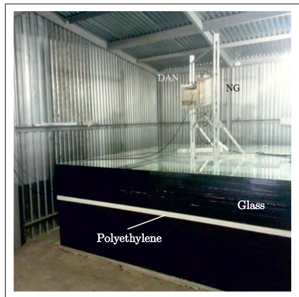
Fig. 19. A planetary soil model with the DAN instrument and neutron generator (NG) above it
