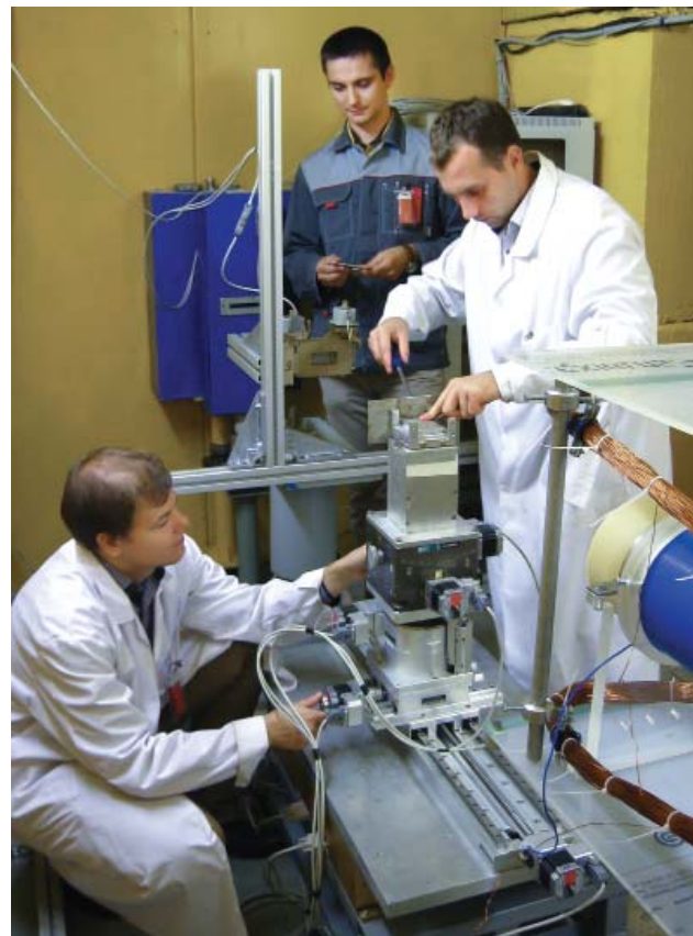
The Frank Laboratory of Neutron Physics. Researchers of the Sector of Neutron Optics adjusting the GRAINS reflectometer. The reflectometric cell of the solid-liquid type where single crystal silicon is used as a substrate is being mounted (Photo by M. Avdeev)
