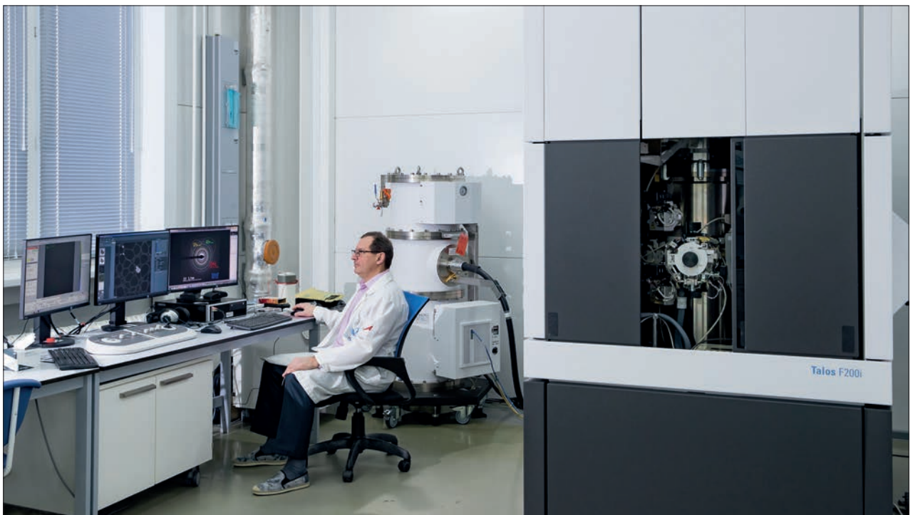
The Flerov Laboratory of Nuclear Reactions. The transmission electron microscope Talos F200i for the study of radiation effects in solids and nanotechnological applications
