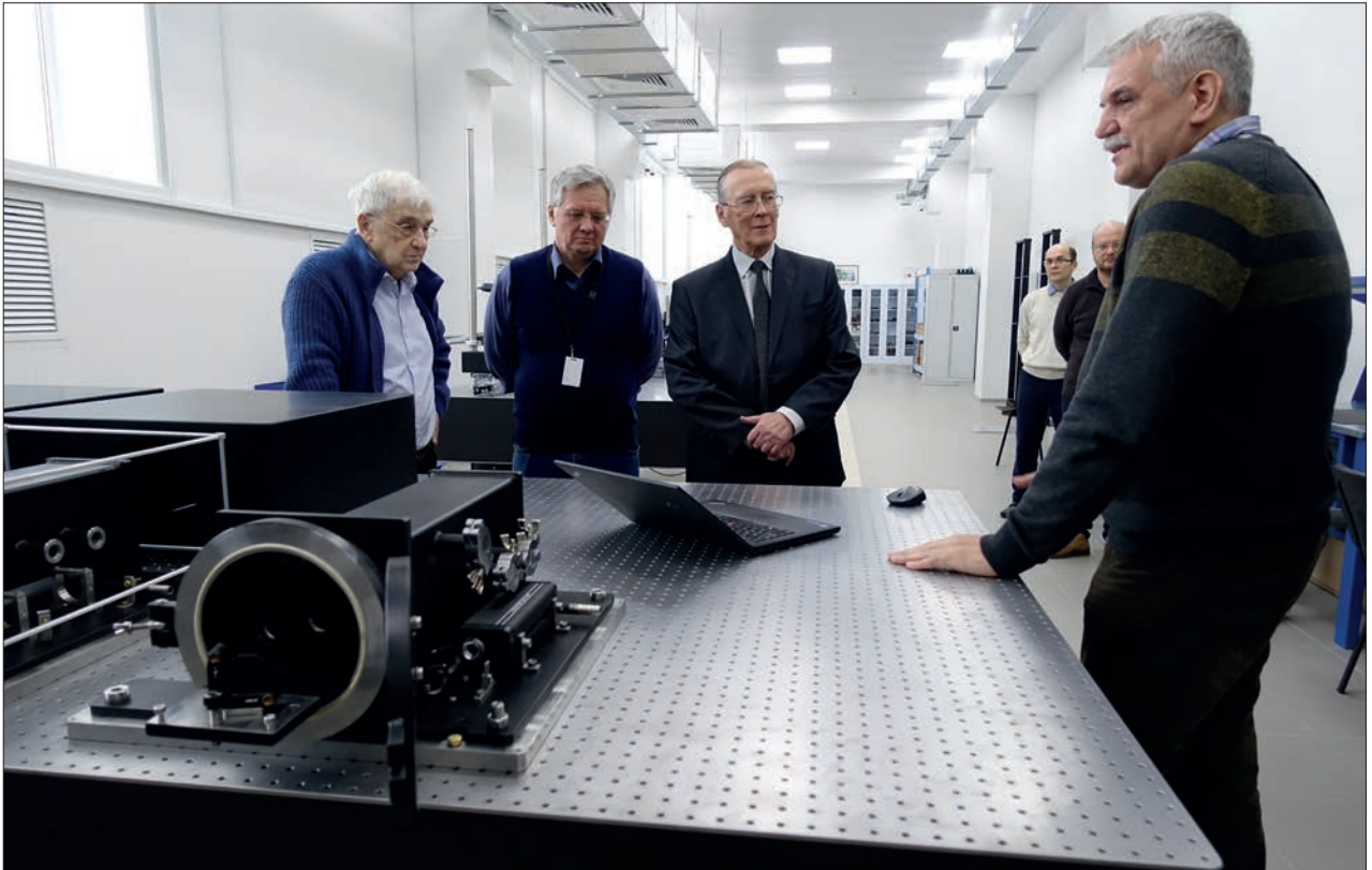
The Dzhelepov Laboratory of Nuclear Problems. The Precision Laser Inclinometer (PLI) — an innovative device for measuring the inclinations of the Earth surface in time with a sensitivity of 2.4 \cdot 10^{-11} \text{ rad/Hz}^{1/2} in the frequency range of 10^{-3} - 12.3 \text{ Hz} . The PLI is currently used at the VIRGO interferometric gravity antenna and at the LHC
