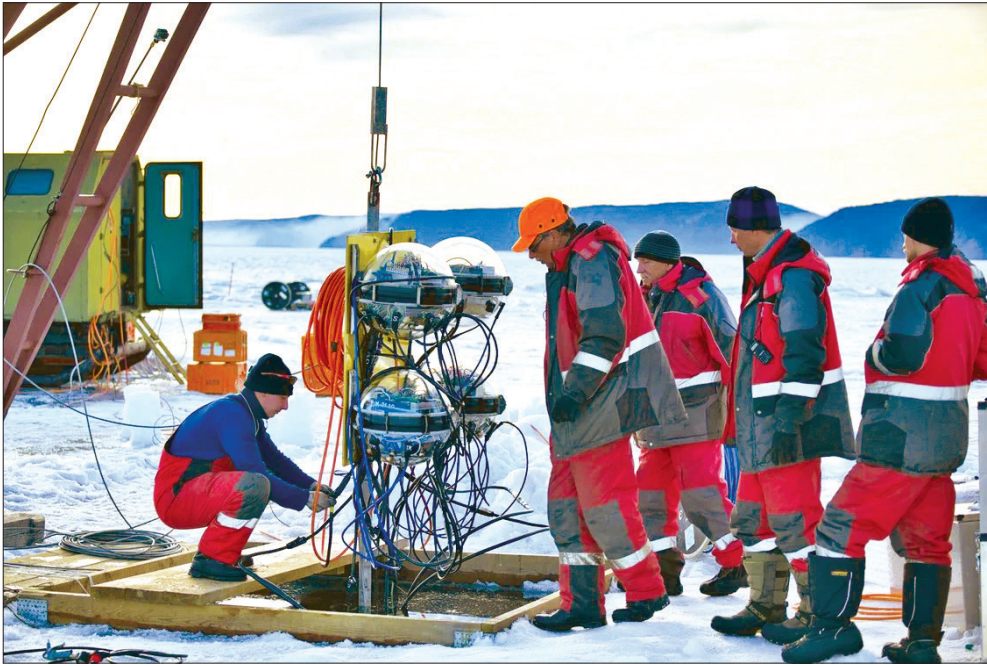
Lake Baikal (Russia). Mounting the central part of the new, seventh cluster of the telescope Baikal-GVD
