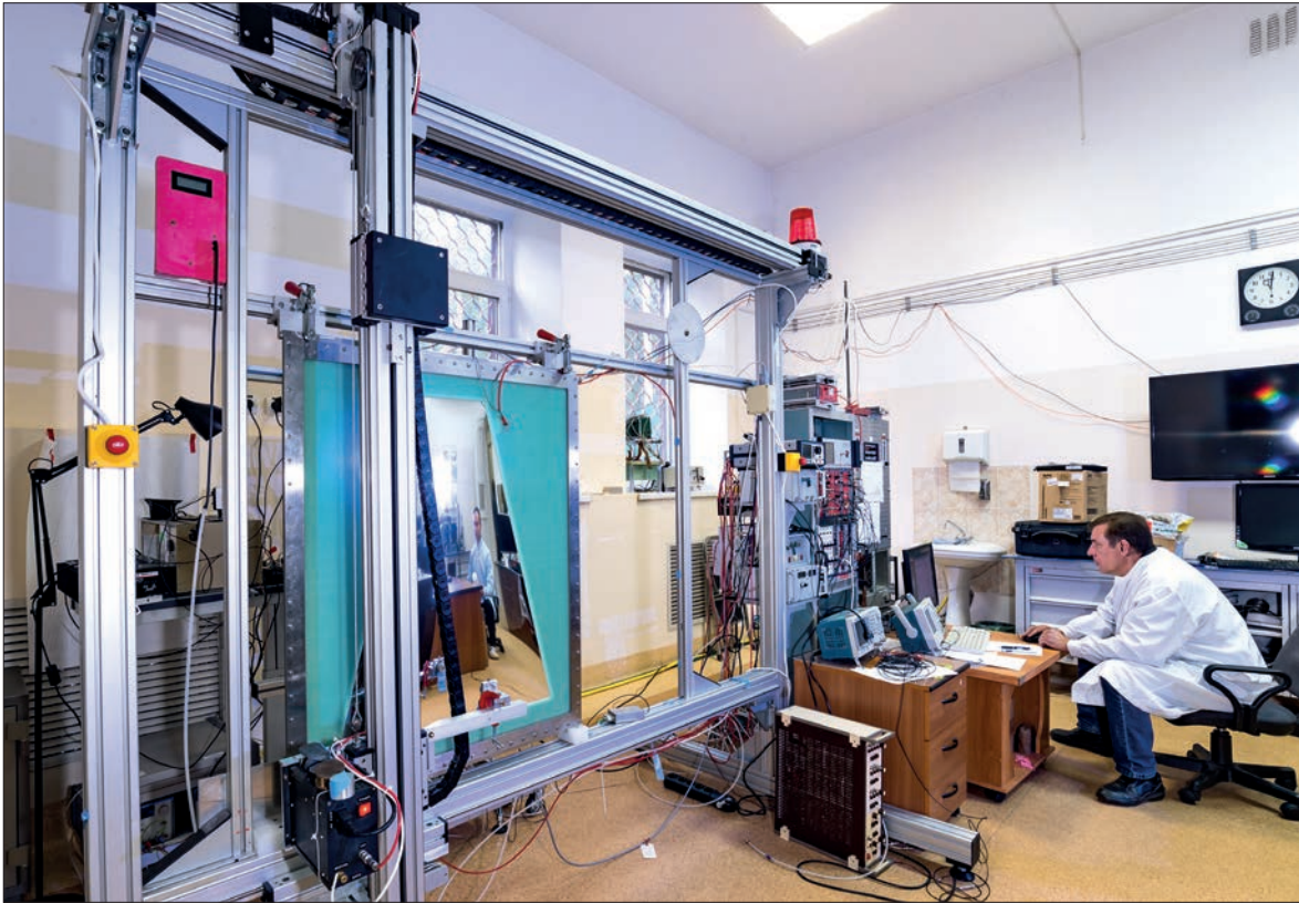
The Veksler and Baldin Laboratory of High Energy Physics. A general view of the automated stand for testing the time projection chamber of the MPD facility
