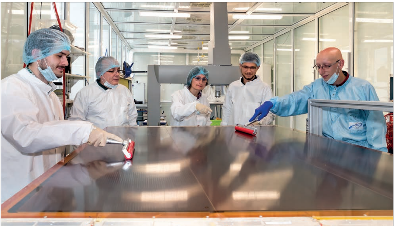
The Dzhelepov Laboratory of Nuclear Problems. Preparation of the read-out panel before the assembling of the Micromegas detector for the ATLAS experiment
