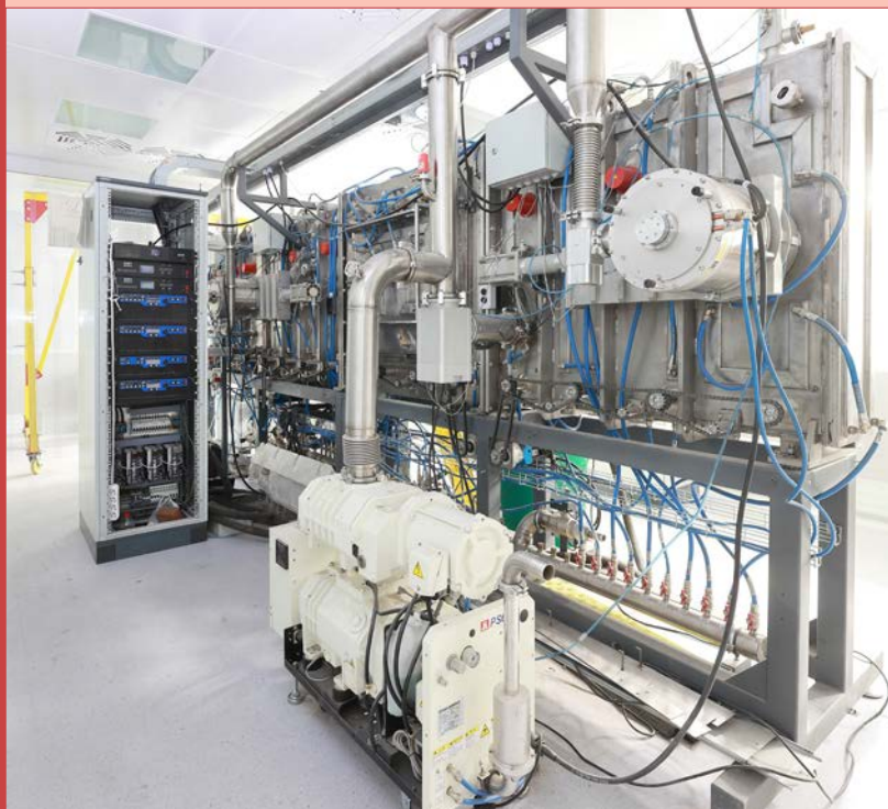
Installation for magnetron sputtering of boron carbide films on substrates made of various materials
