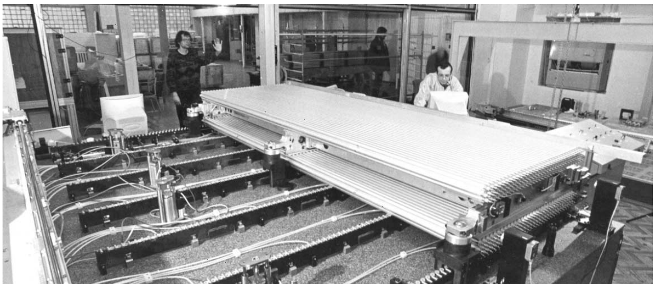
Dzhelepov Laboratory of Nuclear Problems. Area for assembly and tests of drift tubes for CERN's ATLAS experiments
