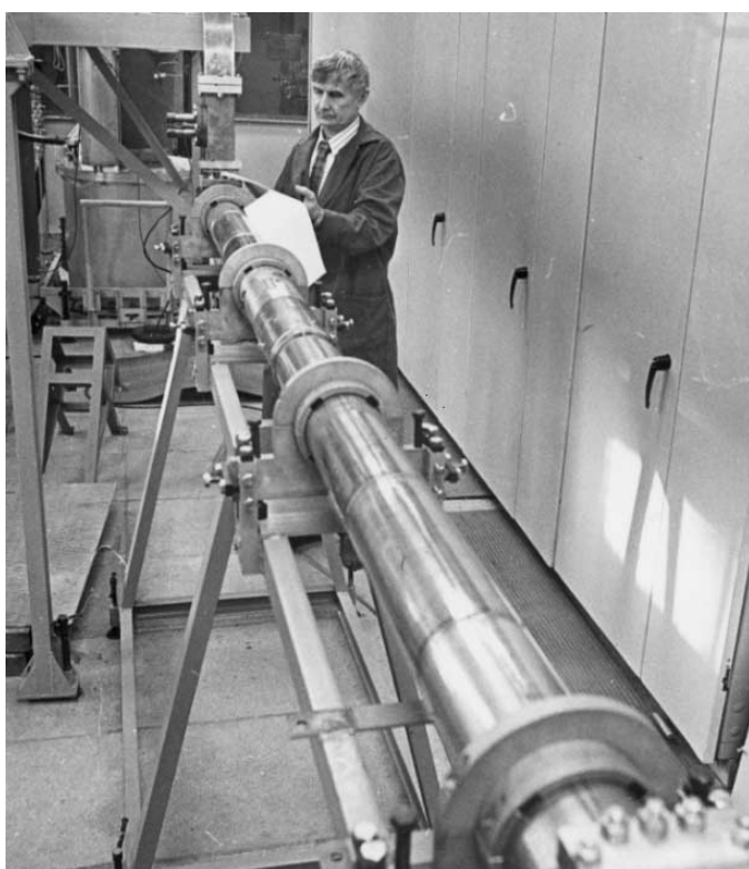
Frank Laboratory of Neutron Physics. SHF-testing of the accelerator section developed at the G.Budker INP (Novosibirsk) for the IREN facility
