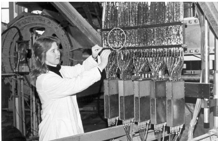
Laboratory of High Energies. The Scintillation Magnetic Spectrometer of Moscow State University (MSU) for joint JINR-MSU investigations into the space-time structure of hadron interactions
