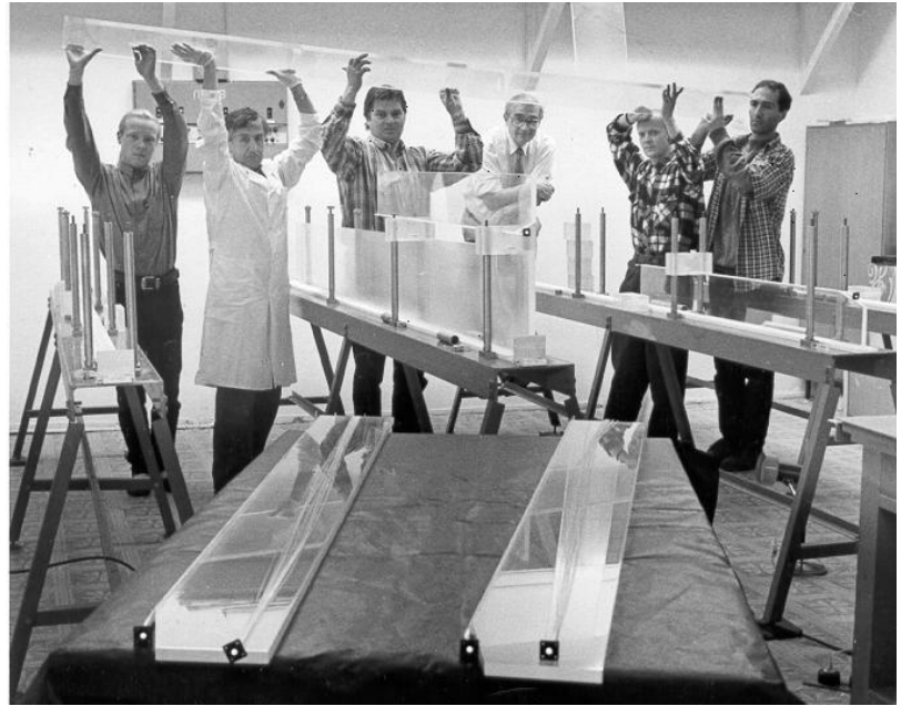
Laboratory of Nuclear Problems. Work under way to construct large scintillator counters for the CDF spectrometry complex upgrade programme at the FNAL Tevatron (USA)
