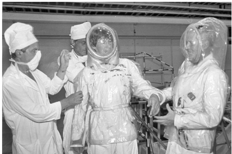
Frank Laboratory of Neutron Physics. Adjustment of protective suits for the IBR-2 personnel to dismantle the reactor's old movable reflector by controlled explosion technique
