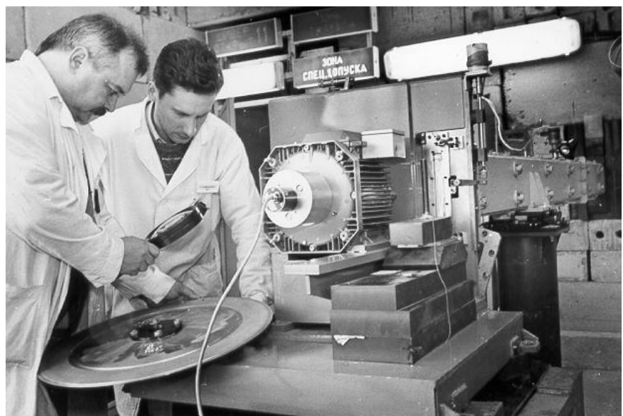
Frank Laboratory of Neutron Physics. Assembling the neutron chopper in the FSD diffractometer purposed for mechanical stress studies in materials
